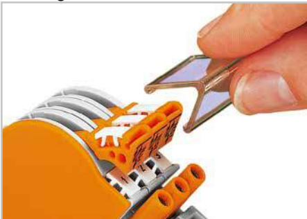
Snapping transparent locking cover onto 1-8 disconnect links: a) Mechanically lock several links for multi-pole switching applications b) Protect markers
