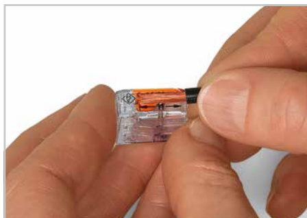
Strip conductor to 11 mm (221 Series). Strip conductor to 9 ... 10 mm (222 Series).
