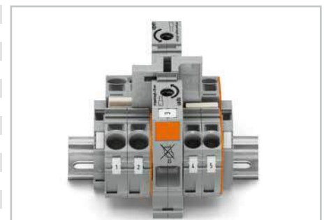
Commoning from 35 mm 2 /AWG 2 POWER CAGE CLAMP terminal blocks to 10/16 mm 2 (AWG 8/10) TOPJOB® S terminal blocks (2010 and 2016 Series)
