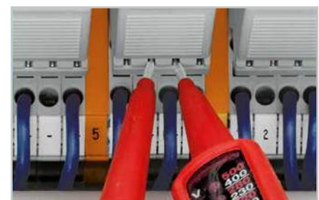
Function testing via touch-proof test slots.
