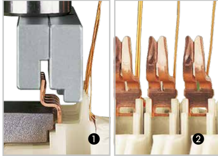
Final assembly of coil contacts: • Pressing in contacts via tool ① • Final position ②
