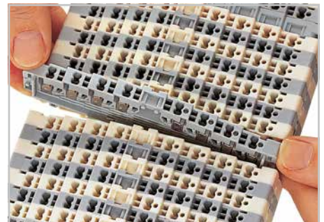
Open the assembly by laterally sliding a block via operating tool (2.5 x 0.4 mm blade). Slide terminal block and remove from the rail with a levering action.
