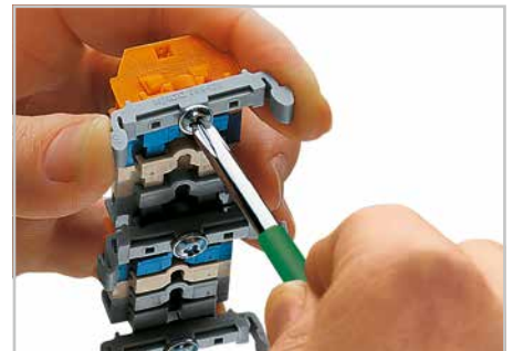
Securing a mounting foot (209-123) to the terminal strip with mounting flanges (distance between mounting feet: approx. 35 ... 40 mm).
