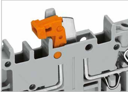
2-conductor disconnect/test terminal block with movable knife disconnect and mechanical interlock – open position
